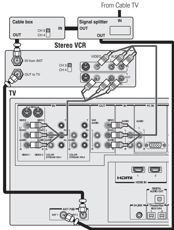
**Note:** The VIDEO/AUDIO OUT terminals output signals from the ANT 1, ANT 2, VIDEO 1, VIDEO 2, and VIDEO 3 terminals when the appropriate input mode is selected.
