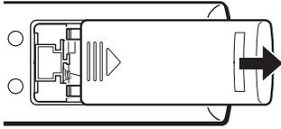
2. Install two “AA” size alkaline batteries. Match the + and – symbols on the batteries to the symbols on the battery compartment.
