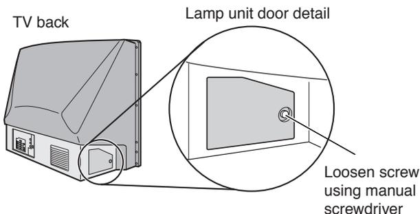
4. Using a manual screwdriver, loosen the two screws on the lamp unit.
